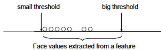
Figure 2.11: The determination of thresholds by weak learner.
